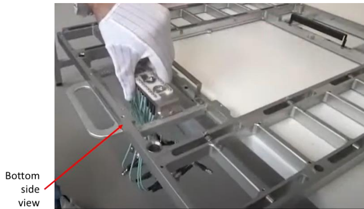
Figure 6: Installing the AT93000-POGO into the loadboard stiffener
